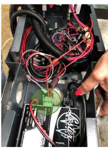
Attach common wire, from battery, into Lockout 2. Attach harness wire, from harness, into Lockout 1.
