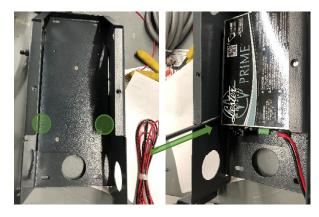
Install lower (2x) #8-32x3/8" pan head machine screws (p/n: 711133) by using a long magnetic philipps-head driver and angling the screw driver as shown.
